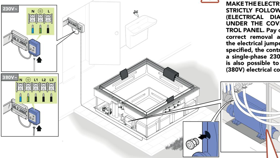
**THE IMAGE SHOWN HERE IS FOR ILLUSTRATIVE PURPOSES ONLY: MAKE THE ELECTRICAL CONNECTIONS STRICTLY FOLLOWING THE DIAGRAM (ELECTRICAL DIAGRAM) PROVIDED UNDER THE COVER OF YOUR CONTROL PANEL. Pay close attention to the correct removal and/or placement of the electrical jumpers. Unless otherwise specified, the control panel is set up for a single-phase 230V connection, but it is also possible to make a three-phase (380V) electrical connection.**
