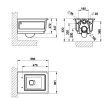
Wall hung WC (6 litres) in Ceramic, integrated siphon. Hardware and lateral holes plugs not included.
