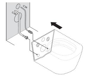
We suggest using the TOTO connecting set SP10695UN for hidden connections WASHLET™ RW, RX, SX GL 2.0, EK 2.0, RG, RG Lite to prepare the water connection on Geberit frames with Sigma concealed cistern 12 cm with empty conduit, located on the left hand side 50 mm from the center of the frame at the same height as the fixation bolts.
