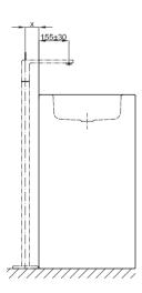
spout projection: distance to wall x mm + ca. 155 mm from outer edge
