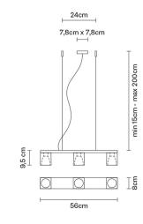
Description Pendant lamp with glass diffusers made of crystal, sandblasted inside. Polished chrome-plated metal structure.
