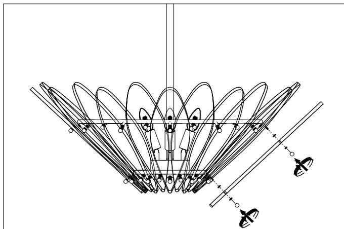
**5.** Place the glass and fix it with the nuts supplied.
