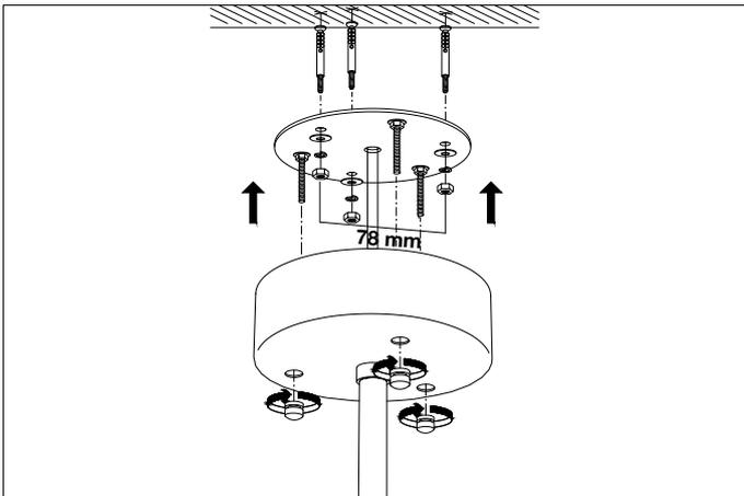
**3.** Fix the bolts to the ceiling. Then fix the ceiling plate to ceiling with screws.
