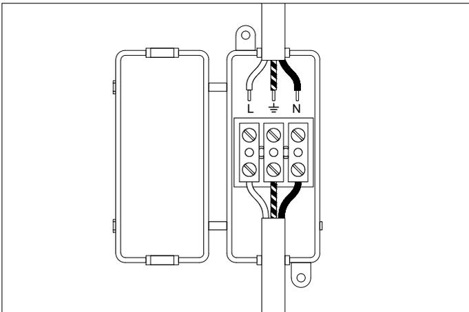
3. Connect the 3 wires according to their colours. Brown is the live wire (L), blue is the neutral wire (N), green/yellow is the earth wire (PE).
