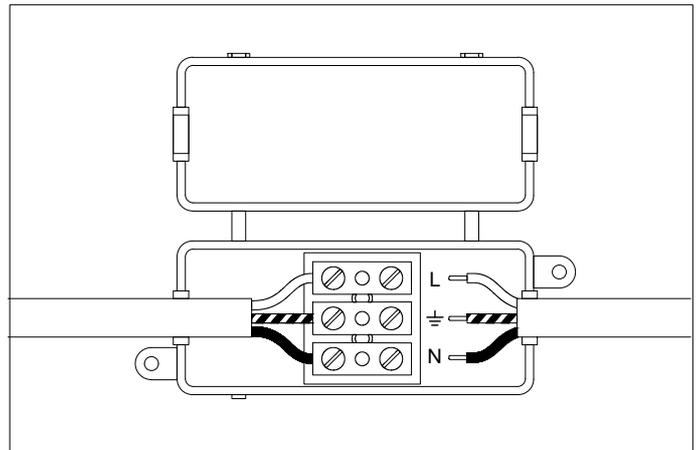
4. Connect the 3 wires according to their colours. Brown is the live wire (L), blue is the neutral wire (N), green/yellow is the earth wire (⊕).
