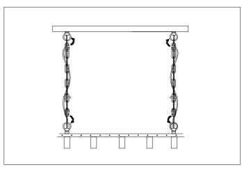
2. Determine the hanging length of the chandelier. Connect the chain according to the height needed. Thread the wires through the chains and ceiling canopy.
