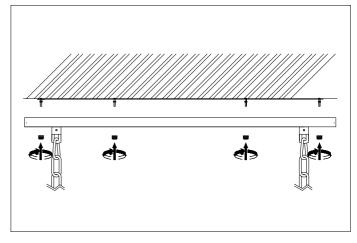
$\boldsymbol{4.}\,\mathsf{Place}$  the canopy over the ceiling plate and fix it with the nuts.
