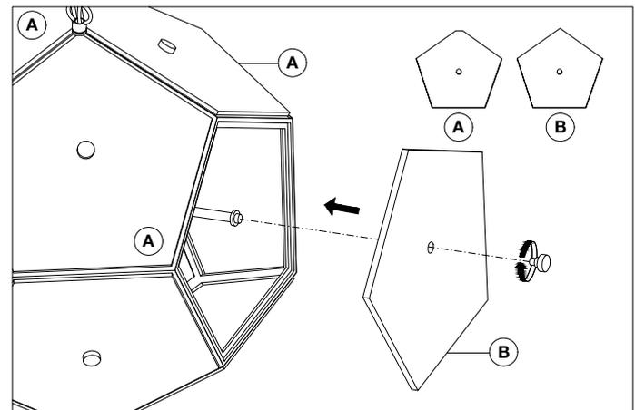
6. Fix the alabaster sheets with the screws supplied. Place the 3 top alabaster sheets (A) and the the bottom alabaster sheets (B).
