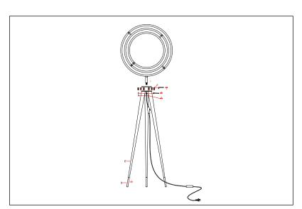
**3.** Connect the tubes and metal plate (C) with screws (6pcs). Then screw the nut and finial.
