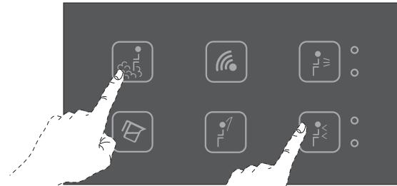
*The control panel shows all keys illuminated with a white light, with reduced intensity.*
