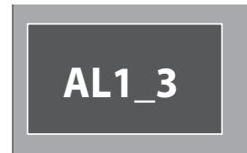
If the errors represented by code "AL1\_X" continue for more than 30 seconds, the relative function/functions (except for the scale removal cycle) will be interrupted.
