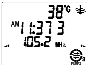
Fig . 11: Radio frequency is 105.2 MHZ, Save the present frequency to channel 3 (Save channel)
