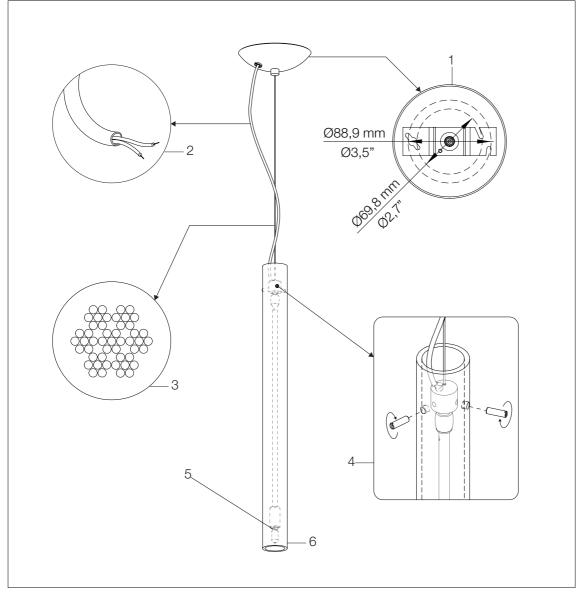
Metal canopy with bracket on the ceiling and measures of distances between holes.
